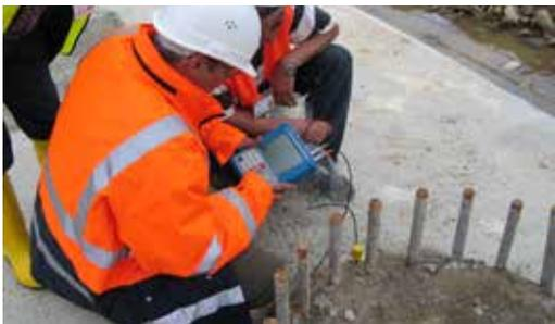
**We are a specialist provider of advanced pile integrity testing services used to assess the condition of concrete pile foundations.**
