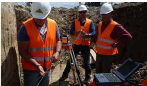
**Cross hole sonic logging provides a full and thorough investigation of the quality and consistency of concrete bored piles.**
