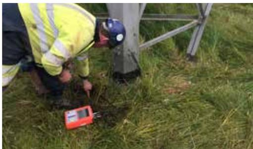
**Using our own specially developed equipment we provide a below ground corrosion assessment service as an alternative method to traditional excavation techniques.**
