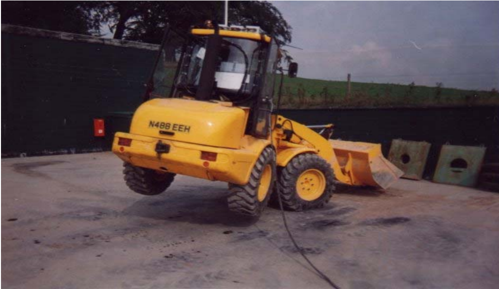
Typical dynamic test of a front shovel machine
