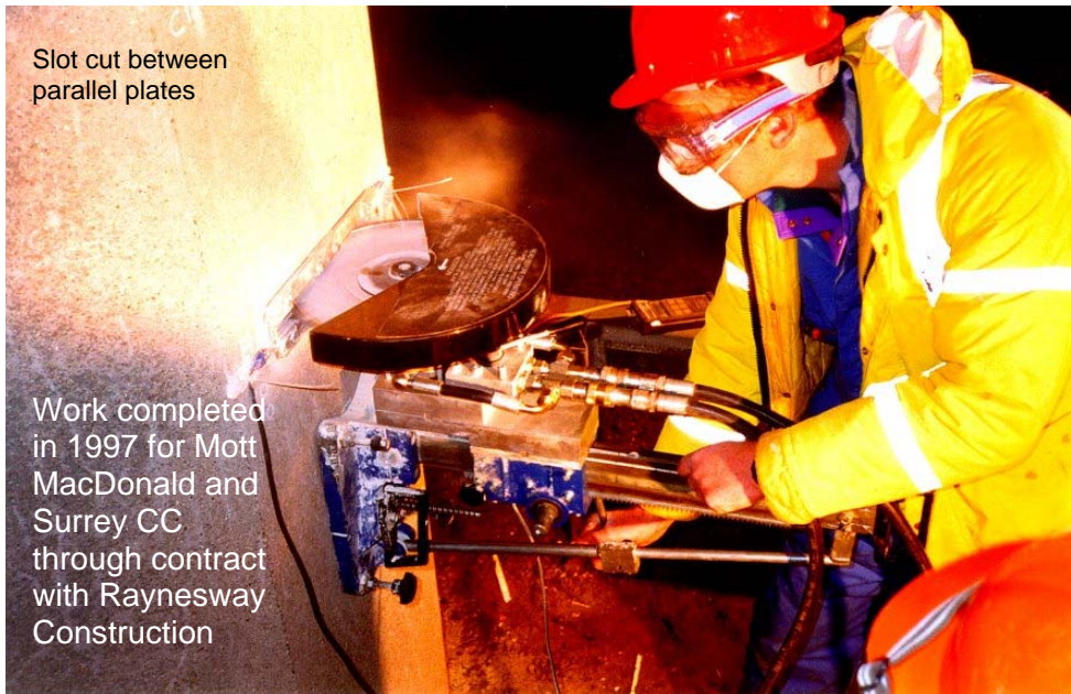
Special jack inserted and pressurised, straingauges monitored
